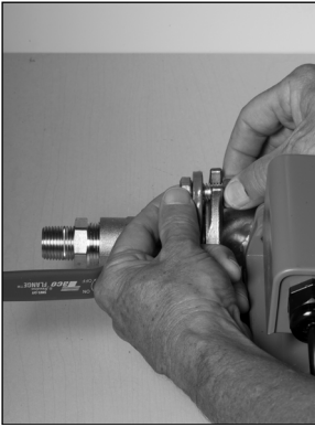
3. Attach shut-off flanges to pump.
