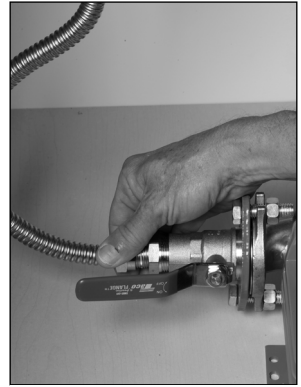
5. Connect flex lines to pump.
